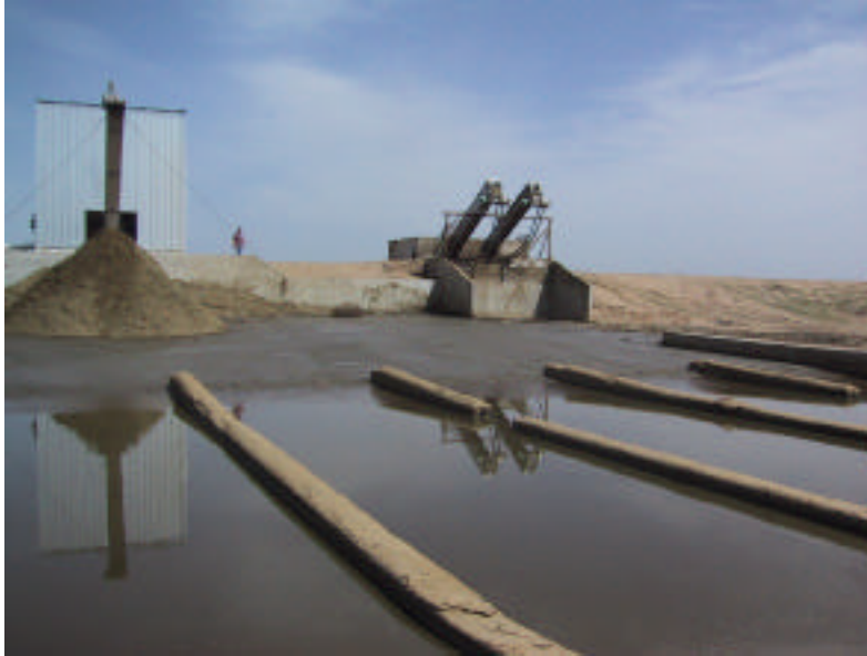
Primary Screens Background with Gravity Separators Foreground
